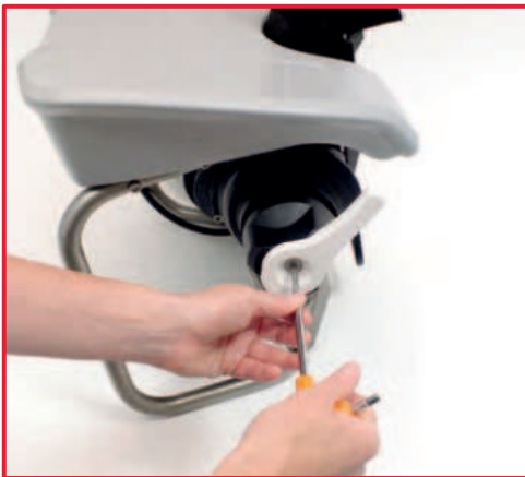
1. Loose the control lever screw.
