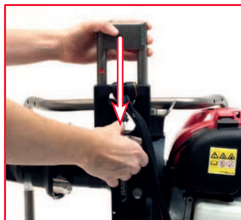
4. Pull open the clamp and slide the short tube into the housing.
