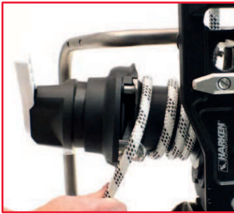
9. Pass the rope over the stripper arm.
