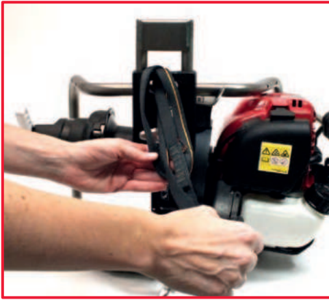
5. Remove the strop from upper anchorage point.
