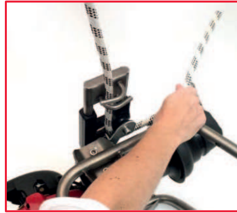
6. Pass the rope round the pulley.
