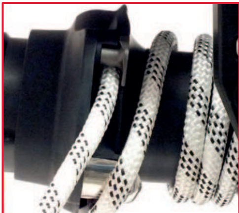
10. Position the rope inside the stopper.
