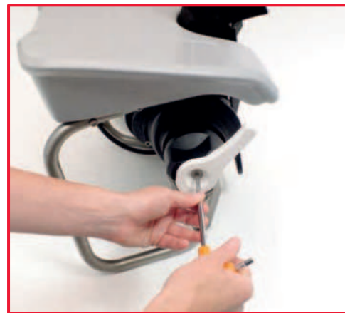
3. Tighten the control lever screw.
