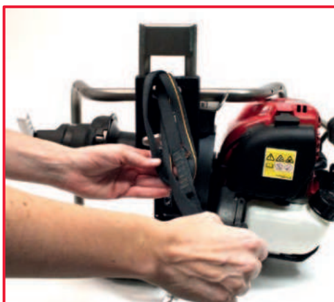
3. Remove the stop from upper anchorage point.
