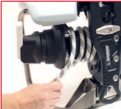
8. Pass the rope over the stripper arm.
