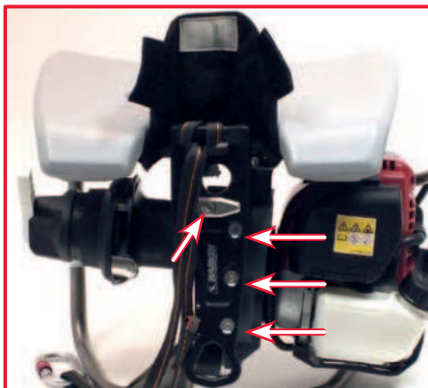
Inspect all screws and check that the marker on the screws and on the plate are aligned. In case of any misaligned contact a HARKEN service center.
