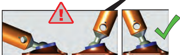
G Correct Position of FLAT Foot The ball joint of the Flat Foot should not be set at its limit of articulation without ensuring that further movement will not occur.
